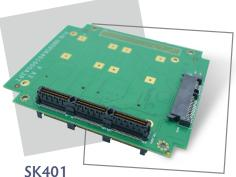
PCIe/104 (StackPC)SSD/mSATA Storage Carrier, Supports 2 x mSATA /mPCIe slots or 1 x 2.5" SATA SSD
