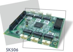
PCle/104(StackPC FPE module) Expand 4 extra 10/100/1000 mbps Gigabit Ethernet
