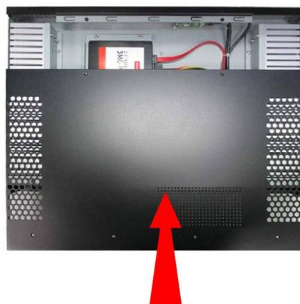
2. Insert one screw in each mounting holes and secure the top case. Use original screws.
